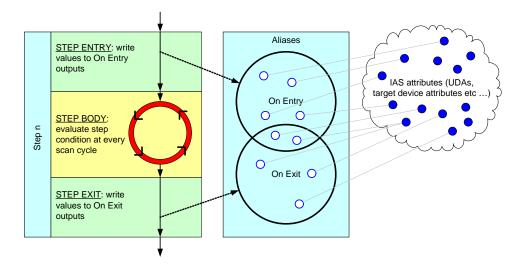
Note Once a step is active, it is evaluated once per scan cycle until it is no longer the active step.
