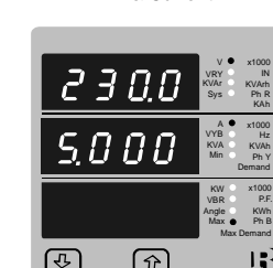
Screen 14 : Max System Voltage & Current
