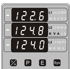
Screen 2 : Phase Apparent power (For 3Phase 4 wire only)
