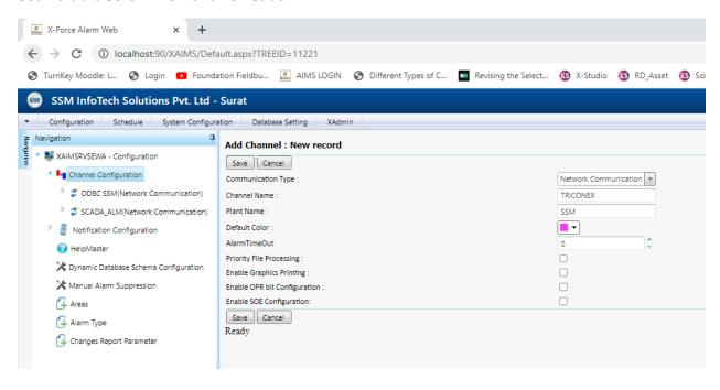
As Shown Below write local IP, Remote IP, Backup IP, Port No, Select Terminator 1 and 2, Set Minimum Length Data accordingly. And click on save.
