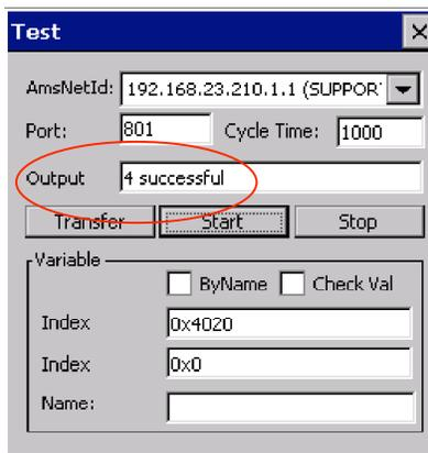
If the results are successful, then your AMS routing information is correct and the connection is ready for use. If the results show any errors, then check your physical cabling and routing information and try again.
