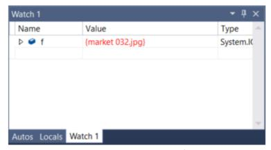
In this example, we have a watch set on the **f** object, and you can see its value change as you move through the debugger. Unlike the other variable windows, the **Watch** windows always show the variables that you are watching (they're grayed out when out of scope).
