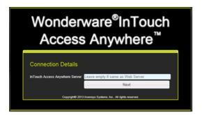
To access InTouch Access Anywhere Server on Node1, enter the machine name or IP address of Node1 in the InTouch Access Anywhere Server field and click Next.
