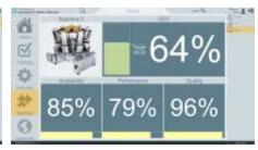
"Andon (Japanese: アンドン or あんどん or 行灯) is a manufacturing term referring to a system to notify management, maintenance, and other workers of a quality or process problem. The center piece is a signboard incorporating signal lights to indicate which workstation has the problem."
