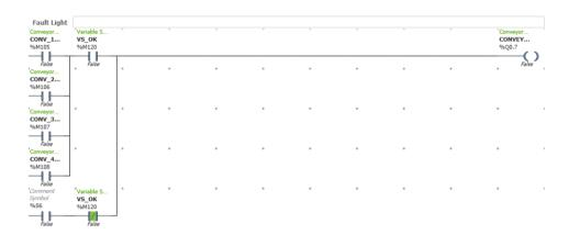
This leg contains %S6 which is the system bit cycling with a 1 second interval. This is in series with **%M120** the normally closed contact is false which is causing the fault light to flash.
