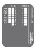
**PWR LED** The first LED shows the state of the power supply to the M221 controller. If the PWR LED is off then the 24V power supply to the M221 is not working. The first thing to check would be the wiring and the power supply itself.
