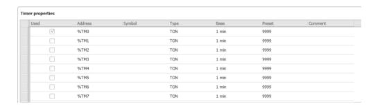
To change the type or base, double-click the column on the row containing the required timer. A drop-down box will appear allowing the type or timebase to be selected.
