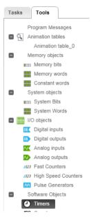
ii. Double-click the **base** column on the row containing **%TM0**. A drop-down box will appear allowing the timebase to be selected. Choose the **1s** (1 second) timebase.
