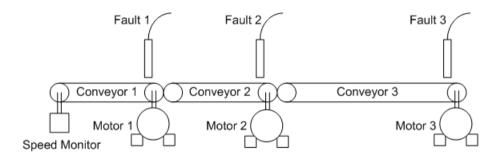
The start control will simply start all three conveyors at the same time although for better control, timers could be used to feed product in a controlled way or distribute startup current for the motors.
