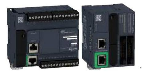
Power supply for all M221 Brick Controllers is by 24VDC connected at the bottom of the unit. The standard M221 Logic Controller can be powered by either 24VDC or 100-240VAC.
