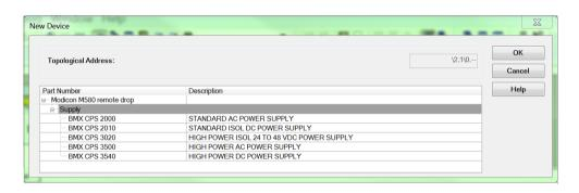
iii. The Power Supply is added to the Rack:
