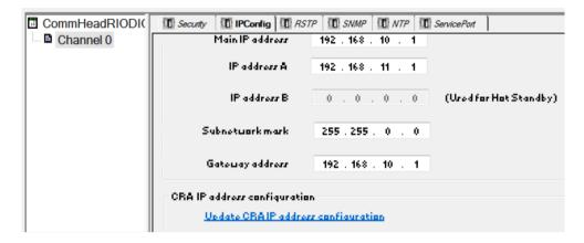
iii. By default the new drop has been added and should be set to IP Address A + 1, if this is not the case change it accordingly. It should be: 192.168.11. 2.
