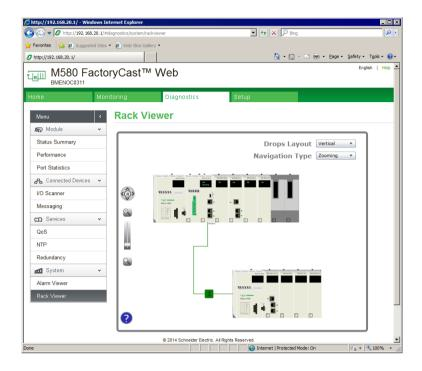
Clicking a module will give detailed information for that module. For example, clicking a NOC module will show Ethernet configuration and port statistics.
