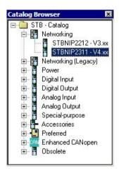
4 To add the **NIM** to the configuration either double-click the **STBNIP2311 - V4.xx** or drag & drop it to the empty island.
