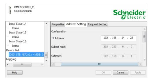
By doing this, the PLC will assign the IP Address 192.168.11.23 to the STB with role name of  ${\tt STBNIP2311\_0XX}$ . To match this name, on the simulator, set the rotary switches on the front of the STB to 3 for ones, and 2 for Tens.
