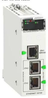
It is functionally similar to the BMX NOC 0402 although it has Cyber Security built in. It also does not require the Interlink cable that is used by the BMX NOC 0401 to communicate with the processor.
