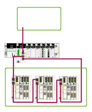
A single connection allows a single device or multiple devices to be "daisy chained" shown above the CPU in the picture above. The configuration shown below the CPU is a Daisy Chain Loop
