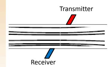
The transit-time is measured from when the transmitter sends the pulse to when the receiver detects the pulse.
