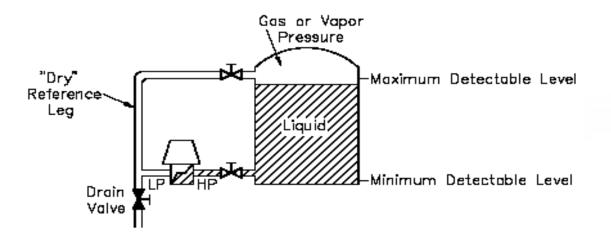
However, if tank is not open to atmosphere then High pressure port is connected to bottom of tank and low pressure port is connected to the top of tank.
