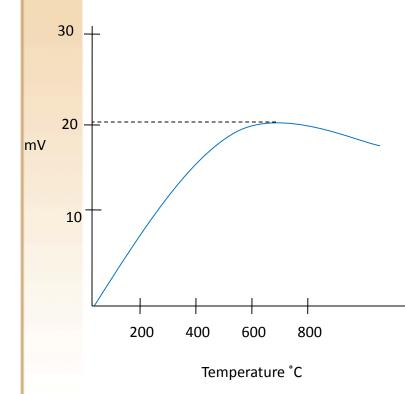
T/C is useful over a limited range of temperature due to non-linear shape of characteristic and reversal that takes after turnover point.
