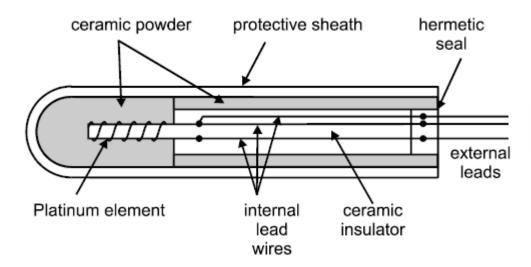
RTD elements are usually long, spring-like wires surrounded by an insulator and enclosed in a sheath of metal.
