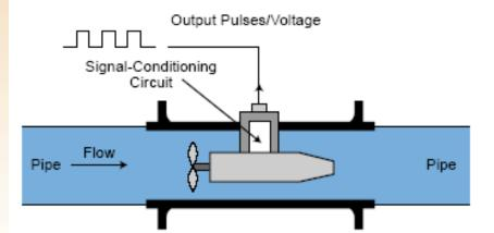
Magnetic pick-up or inductive proximity switch detects the rotor blades as they turn.
