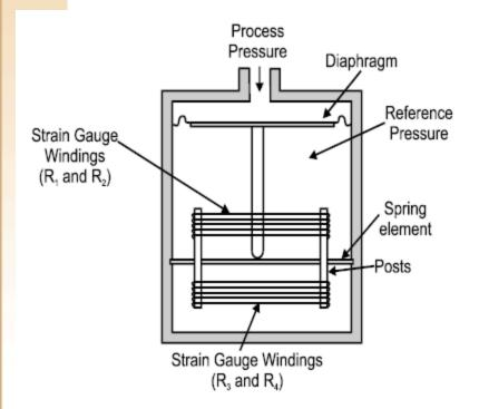
Typically, four strain gauges are bonded to a metal or plastic flexible diaphragm and connected into a Wheatstone bridge circuit
