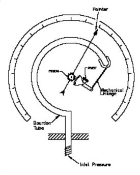
The tube is bent lengthwise into an arc of a circle of 270 to 300 degrees.
