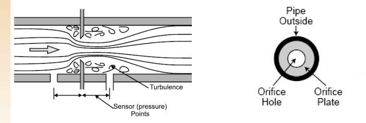
A standard orifice plate is simply a smooth disc with a round, sharp-edged opening in center.
