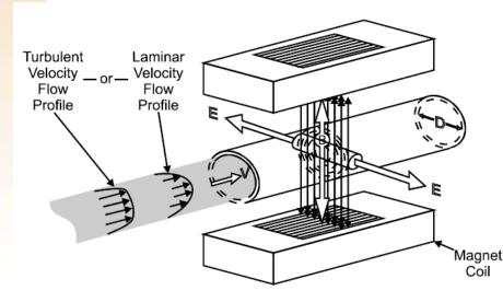
A conductive liquid consisting of charged particles will then produce a voltage proportional to the volumetric flow rate.
