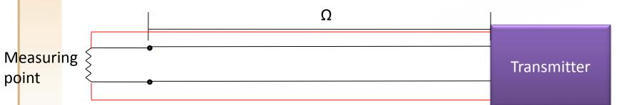
To compensate this error extra wire is connected from measuring point to transmitter.
