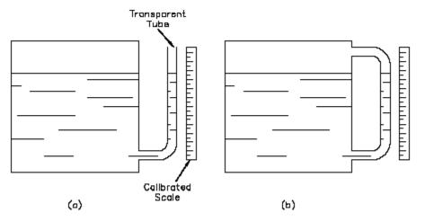
In the gauge glass method, a transparent tube is attached to the bottom and top of the tank that is monitored.
