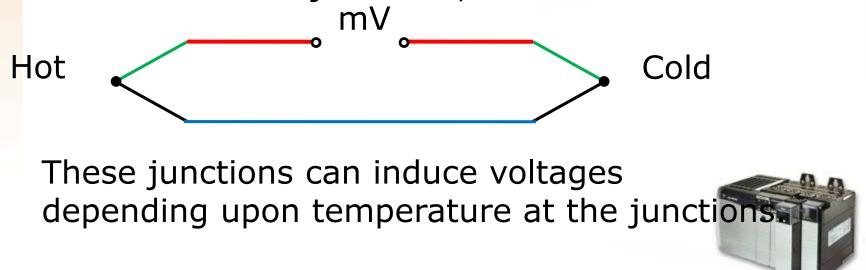
Secondly, Reference junction temperature should be constant and ideally should be 0 °C for accurate measurement, but it is never.
