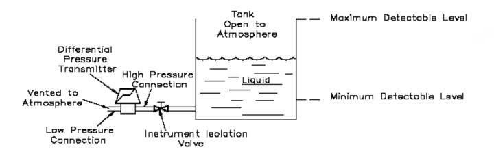
Pressure Measured is proportional to the amount or level of liquid in the tank.
