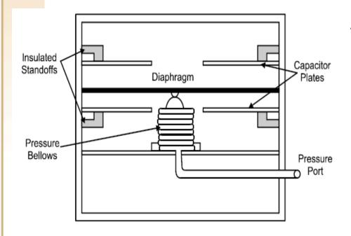
As the diaphragm is deflected due to pressure changes, the relative capacitance is measured by a bridge circuit.
