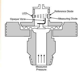
The received light on the measuring diode indicates the position of the diaphragm.
