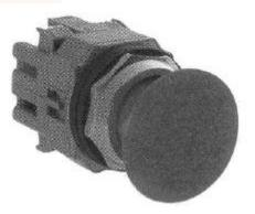
Detent pushbutton are known as Emergency Stop of E-Stop When pressed in it remains in, and then to return it to its original position, it must be pulled o
